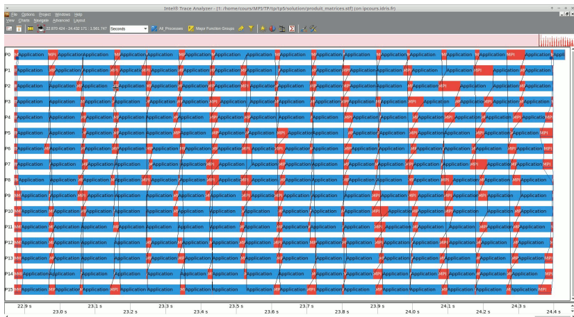
Figure 28 – Parallel matrix product on 16 processes, for a matrix size of 1024 (second algorithm)
